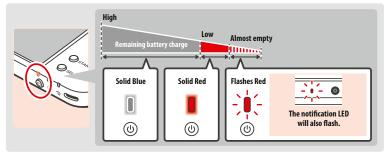
Note: If the power LED is red, save your game quickly and recharge. If the battery charge runs out before you save, you may lose unsaved data. If the LED is blue and slowly brightens and dims, the system is in Sleep Mode (2 p. 15), which will conserve battery power.
